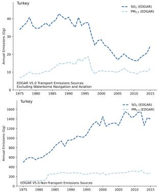
Figure 46: Transport (left) and non-transport (right) emissions of SO<sub>2</sub> and PM<sub>2.5</sub> in Turkey
