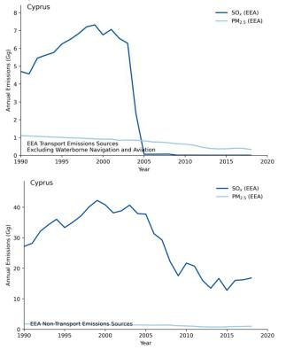
Figure 14: Transport (left) and non-transport (right) emissions of SO<sub>X</sub> and PM<sub>2.5</sub> in Cyprus
