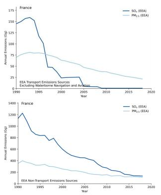
Figure 18: Transport (left) and non-transport (right) emissions of SO<sub>X</sub> and PM<sub>2.5</sub> in France
