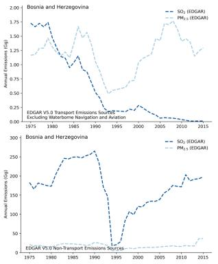
Figure 9: Transport (left) and non-transport (right) emissions of SO<sub>2</sub> and PM<sub>2.5</sub> in Bosnia and Herzegovina
